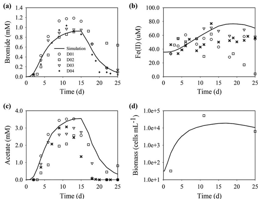
**FIG 1** (a to c) Simulated (solid line) and observed (symbols) bromide breakthrough (a), Fe(II) breakthrough (b), and acetate breakthrough (c) at the first row of monitoring wells D01, D02, D03, and D04. (d) Comparison of *Geobacter* response from the simulation (solid line) and the qPCR data (open squares) at downgradient monitoring well D02 in Chandler et al. (11).
