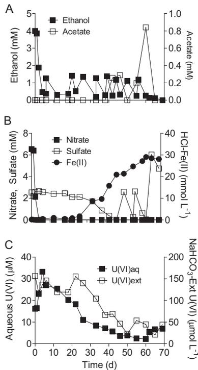
**FIG 1** Concentrations of ethanol, acetate, nitrate, sulfate, 0.5 M HCl-extractable Fe(II), aqueous U(VI), and NaHCO<sub>3</sub>-extractable U(VI) during the initial phase of the sediment slurry experiment designed to drive the slurries into sulfate-reducing conditions.
