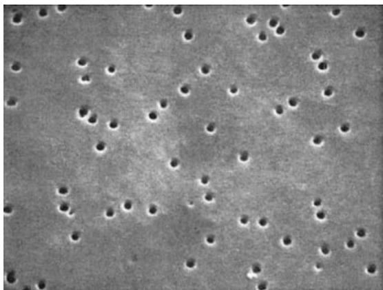
**Figure 12.4.4** Scanning electron micrograph (10 000×) of the surface of a 0.2- $\mu\text{m}$  pore-size polycarbonate track-etch membrane filter.
