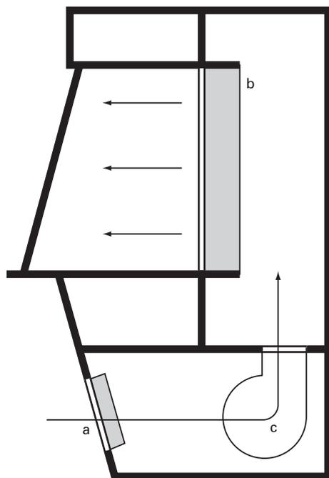
**Figure 12.4.12** Horizontal laminar-air-flow unit. (a) Prefilter; (b) HEPA filter; (c) fan.
