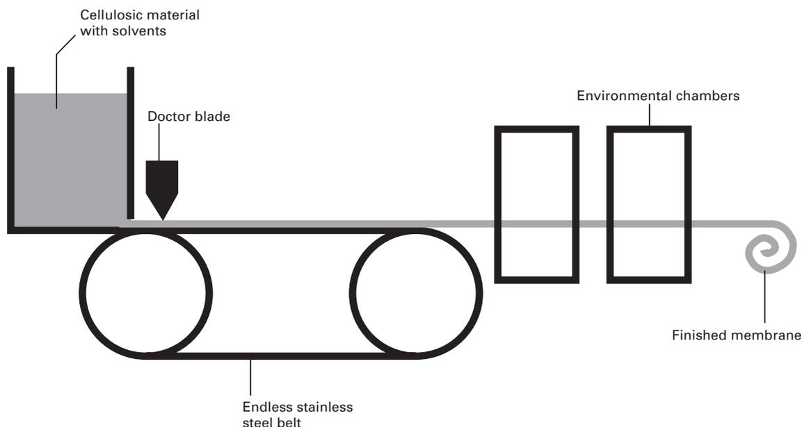
**Figure 12.4.1** Membrane manufacture – the casting process.
