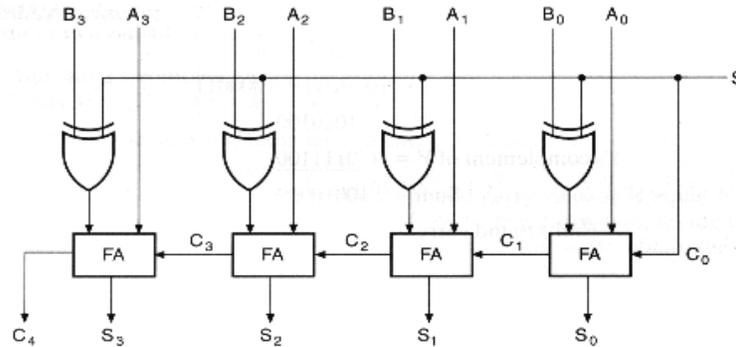
Figure (5) 4-bit binary adder/subtractor circuit
