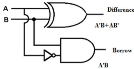
Figure (2) Logic diagram of half-subtractor
