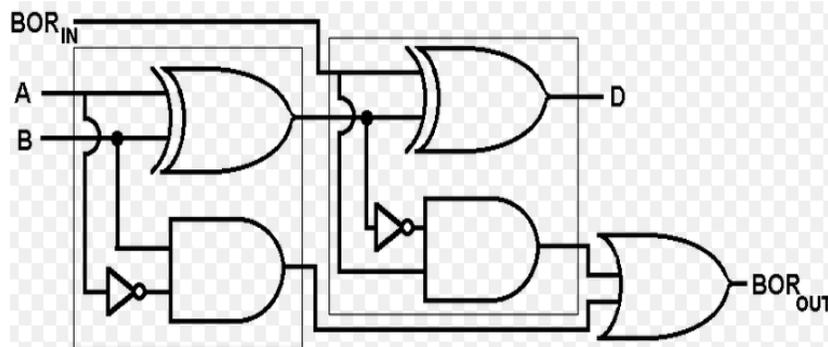
Figure (4) Logic diagram of Full-subtractor
